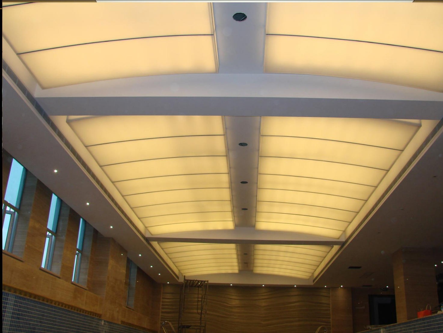
C. Translucent Film use with fluorescent tube
